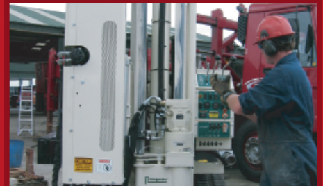
Automatic SPT Drop Hammer
